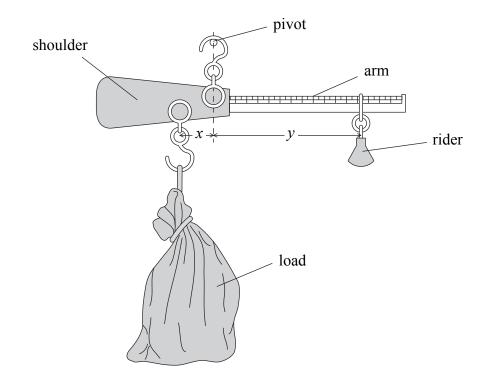
The weight of the shoulder balances the weight of the arm. The weight of the rider is  $8.0 \,\mathrm{N}$  and this balances the weight of the load when  $x = 0.12 \,\mathrm{m}$  and  $y = 0.60 \,\mathrm{m}$ .
